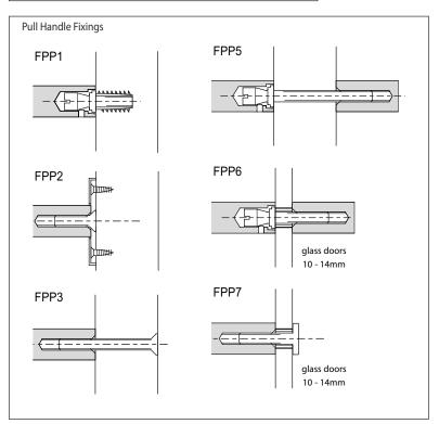
Note: All bolts are M8. Clearance hole for glass door fixings -  $14\text{mm}\,\text{Ø}$
